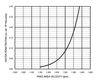
The AMCA Water Penetration Test provides a method for comparing various louver models and designs as to their efficiency in resisting the penetration of rainfall under specific laboratory test conditions. The point of zero water penetration is defined as that velocity where the water penetration curve projects through .01 oz of water penetration per sq. ft. of louver area. The beginning point of water penetration for AC-660 is 1,151.3 fpm free area velocity.
