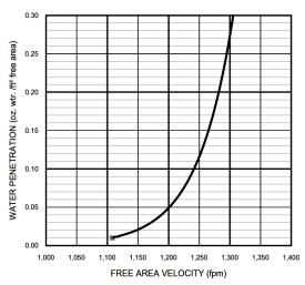
The AMCA Water Penetration Test provides a method for comparing various louver models and designs as to their efficiency in resisting the penetration of rainfall under specific laboratory test conditions. The point of zero water penetration is defined as that velocity where the water penetration curve projects through .01 oz of water penetration per sq. ft. of louver area. The beginning point of water penetration for RSR-900 is 1,108 fpm free area velocity.
