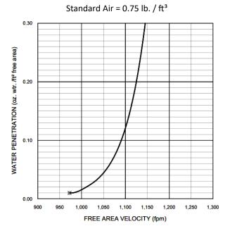
The AMCA Water Penetration Test provides a method for comparing various louver models and designs as to their efficiency in resisting the penetration of rainfall under specific laboratory test conditions. The point of zero water penetration is defined as that velocity where the water penetration curve projects through .01 oz of water penetration per sq. ft. of louver area. The beginning point of water penetration for DL-440 is 973 fpm free area velocity.
