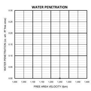
The AMCA Water Penetration Test provides a method for comparing various louver models and designs as to their efficiency in resisting the penetration of rainfall under specific laboratory test conditions. The point of zero water penetration is defined as that velocity where the water penetration curve projects through .01 oz of water penetration per sq. ft. of louver area. **The beginning point of water penetration for RSR-545VPF is 1250 fpm free area**
